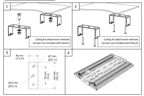
Attach the ceiling brackets to the installation surface.
