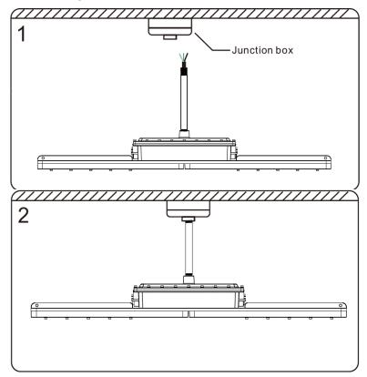
The pendant conduit should be screwed-in by at least 6 threads.
