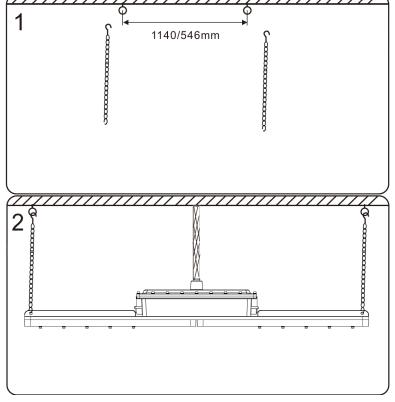
Drill 2x holes for hanging rings (546mm apart for 2-ft fixtures, 1140mm apart for 4-ft fixtures)
