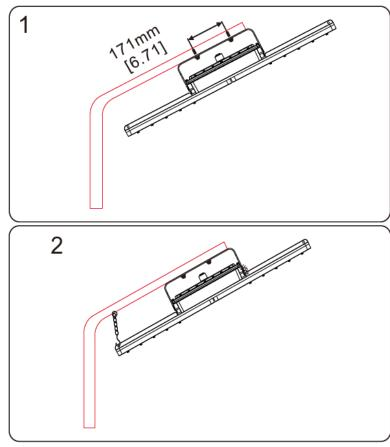
Drill 2x Ø15mm holes for fixture the screws
