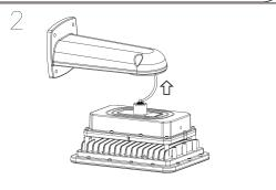
Connect the AC power with fixture
